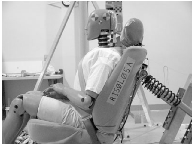
Figure 1. Test setup of a 50 th percentile dummy positioned in the test seat on a deceleration sled
