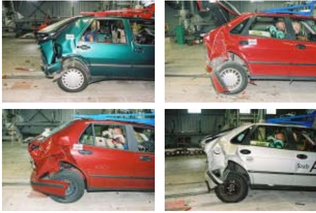
Figure 7: Vehicle static crush with 48.3 km/h barrier speed. The top left is the Saab 9000, top right Saab 900, bottom left the Saab 9-5 and bottom right the Saab 9-3.
