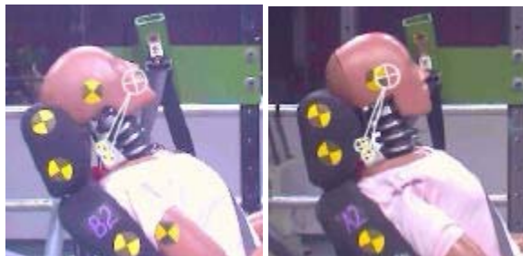
Figure 4: Kinematics of the Hybrid III dummy in rear sled tests with a superimposed reference target on the clavicle showing the initial head position in a moving reference frame fixed to T1. The peak head displacement and extension angle are shown with respect to T1. The left picture shows the peak head displacement for the baseline luxury seat and the right, the same seat with SAHR integrated into the seatback.
