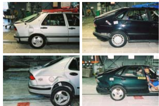
Figure 6: Vehicle static crush with 24.0 km/h barrier speed. The top left is the Saab 9000, top right Saab 900, bottom left the Saab 9-5 and bottom right the Saab 9-3.
