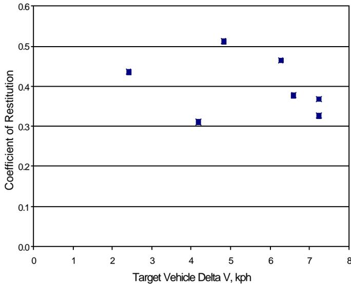
Figure 1. Coefficient of Restitution v. Target Vehicle Delta V, kph
