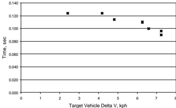
Figure 2. Duration of Impact v. Target Vehicle Delta V, kph
