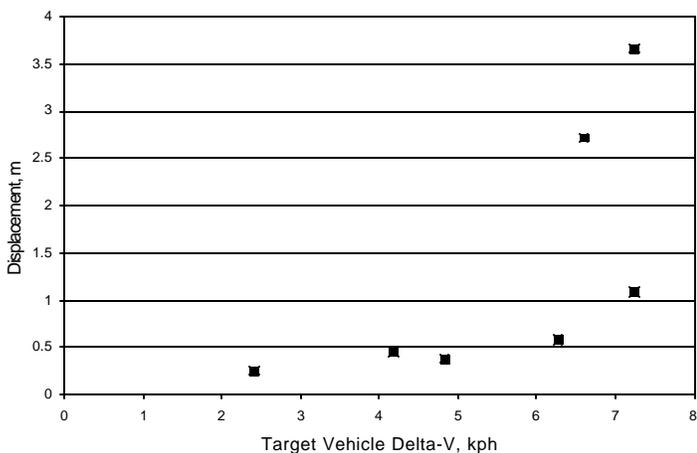
Figure 4. Target Vehicle Forward Displacement Results
