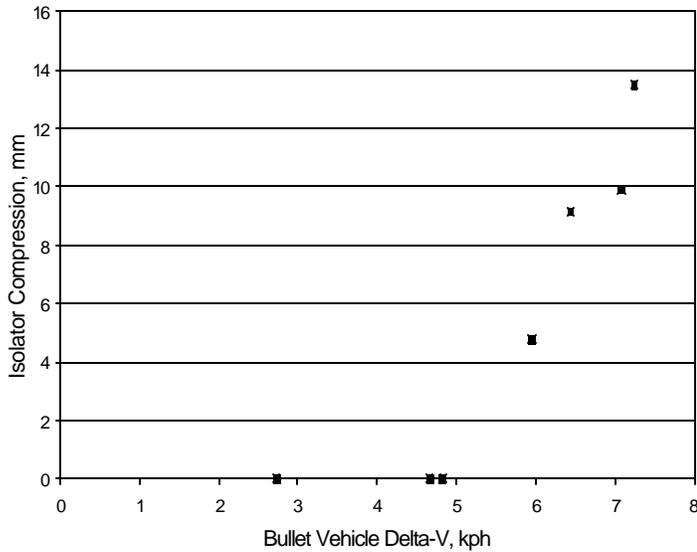
Figure 3. Bullet Vehicle Isolator Compression Results
